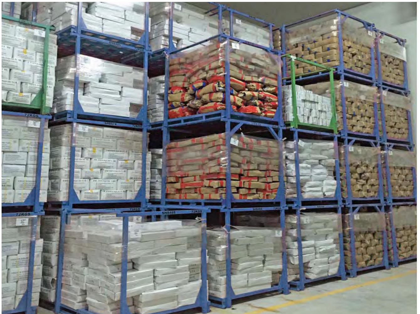
Special made - design for stack 4 pallet cages
